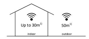
CASAMBI uses the MESH network technology. Each device acts like a repeater and refreshes the received Bluetooth signal for the following devices.
