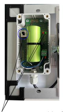
Switch to off means that the antenna is not active and therefore there is no deep discharge of the battery.
